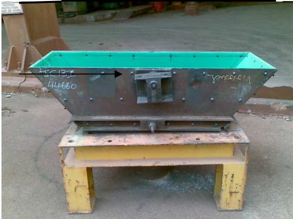
Photo 003 – Side view of similar adjacent U034313 chute showing attachment of pivot bracket
