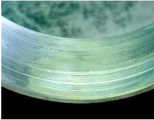
This Bearing Showed Evidence of Spalling on the Bearing After 18,000 Hours
