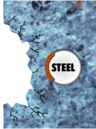
Remove spalled concrete from deteriorating structure.
