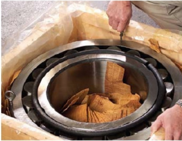
Fig. 2 Eyebolts can be inserted into lifting holes
